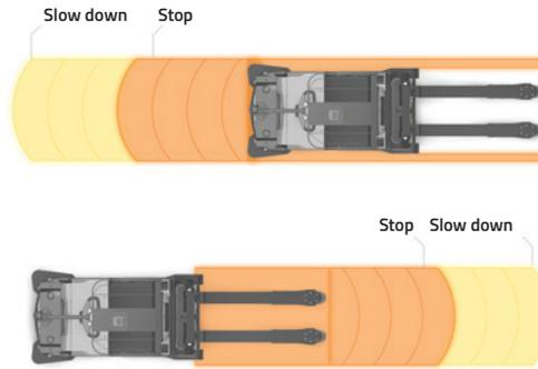
Front and rear scanners for safe transportation at rated speed
