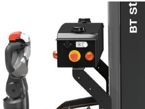
E-stop buttons easily reachable for operators in workplace
