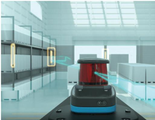
Reflector navigation is a navigation method in which consistent and high-contrast targets, reflectors, are added to the environment. The reflectors installed in the warehouse allow the scanner on the automated truck to define its position based on its distance to the reflectors. The characteristics of this technique guarantee robustness, high accuracy and long reach in most environments.
