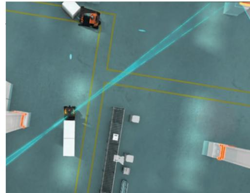
Natural navigation is an alternative navigation technique for warehouses where the surroundings remain fairly constant. The truck can utilise the existing environment to navigate without reflectors, avoiding extra cost and additional equipment. A unique benefit from Toyota is the fact that the Autopilot can switch seamlessly between natural and reflector navigation depending on the area it's in - we call this dual navigation.
